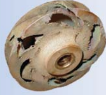
Above: cavitated impeller from commercial pool pump
